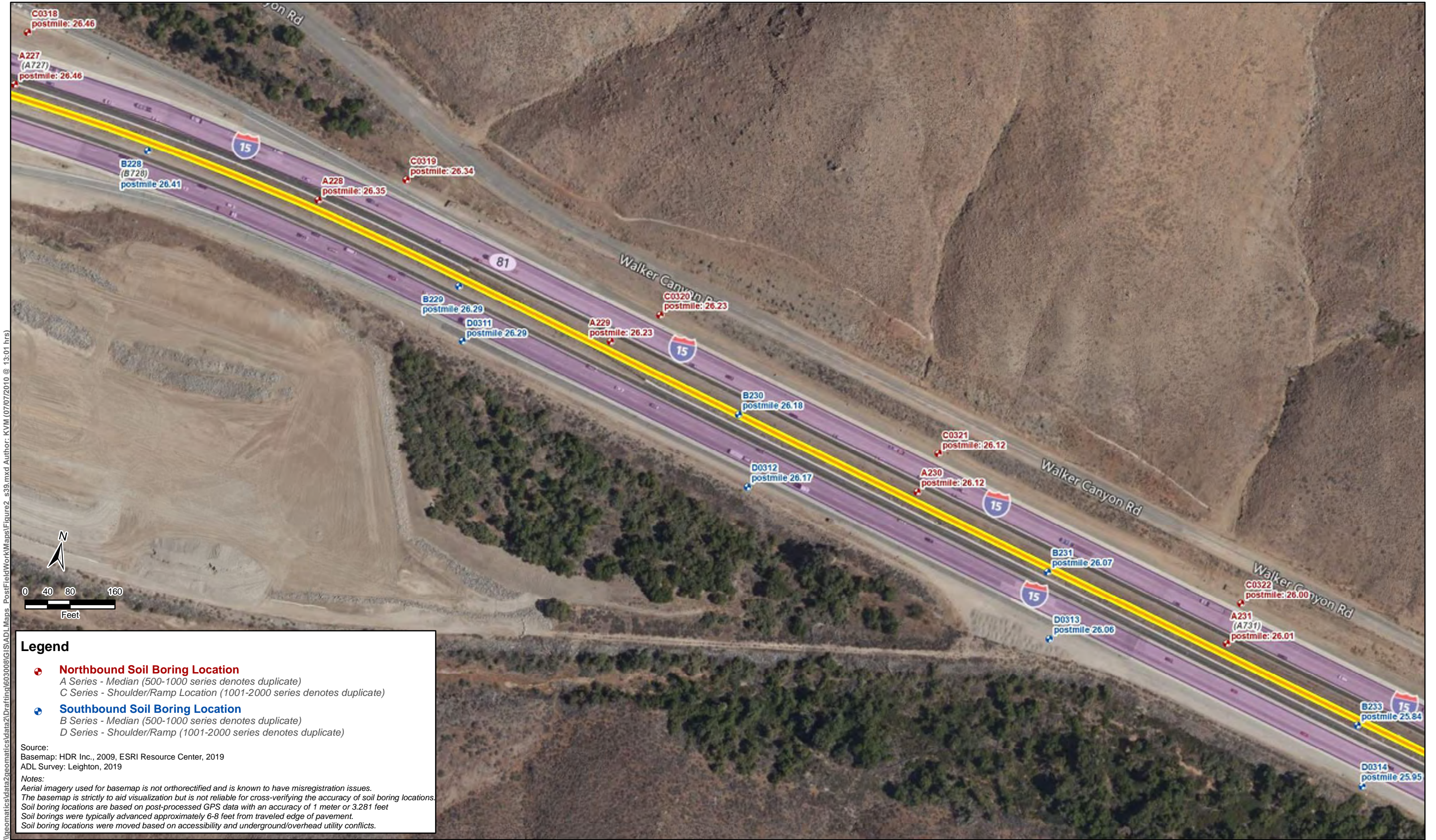
Figure 2 (s14) Boring Location Map, Aerially Deposited Lead Survey I-15 Corridor Improvement Project, Riverside County, California
