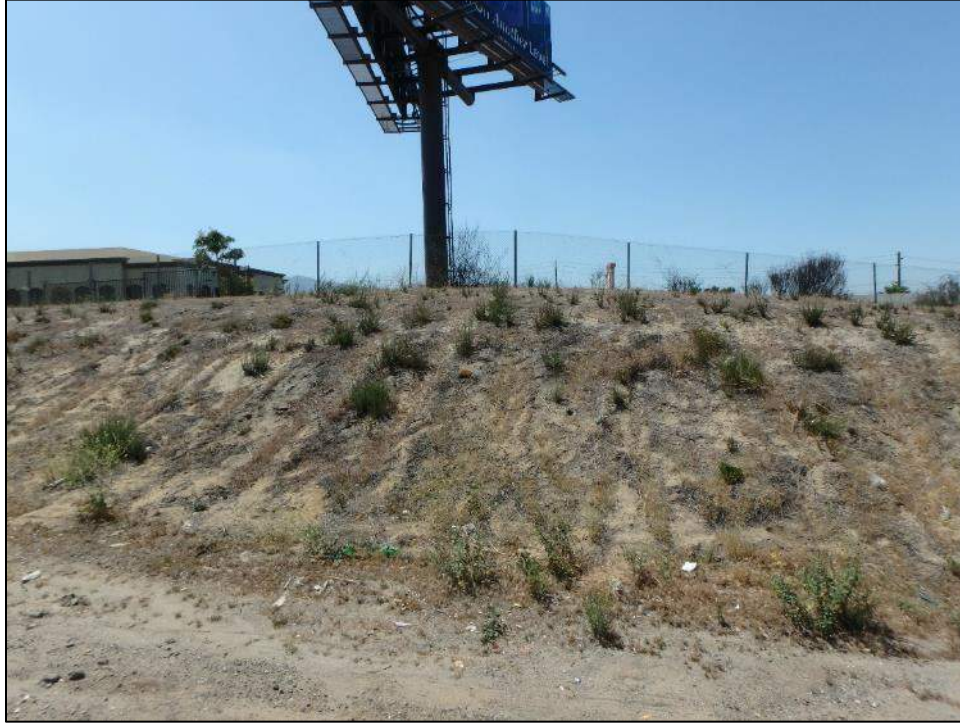
Photo 17. Outcrop exposure of late to middle Pleistocene-age old alluvial fan deposits (Qof) on the shoulder along the northern section of the survey area. View to the west.
