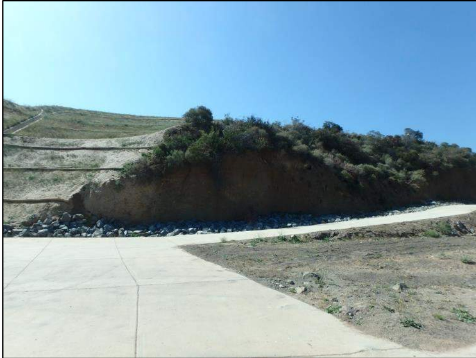
Photo 11. Overview of sediment exposure above Bedford Wash containing late to middle Pleistocene-age old alluvial fan deposits (Qof). View to the south.
