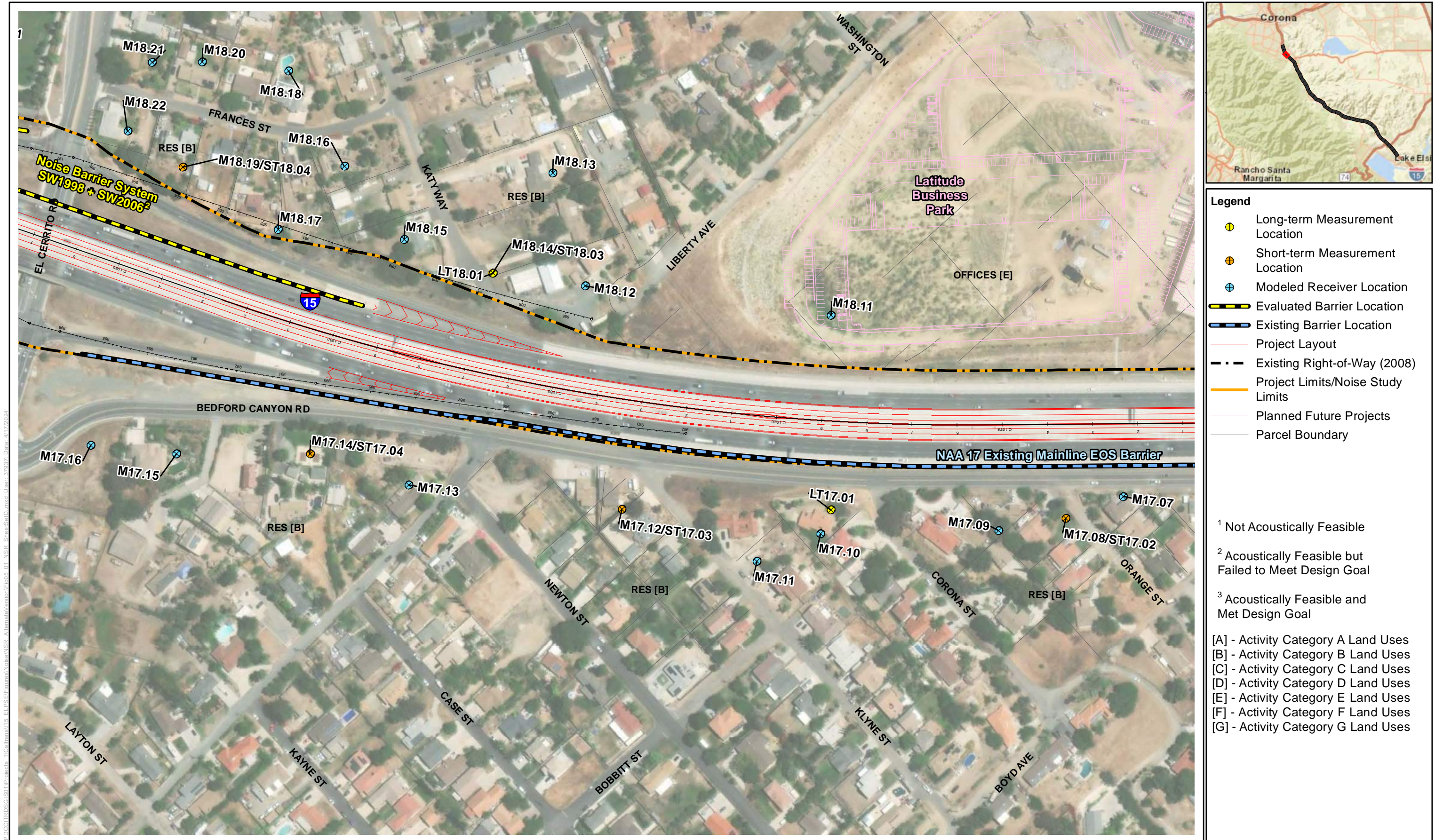
Figure 5-1, Sheet 38d of 40 Noise Measurement and Modeling Locations, and Evaluated Noise Barriers Interstate 15 Express Lanes Project Southern Extension
