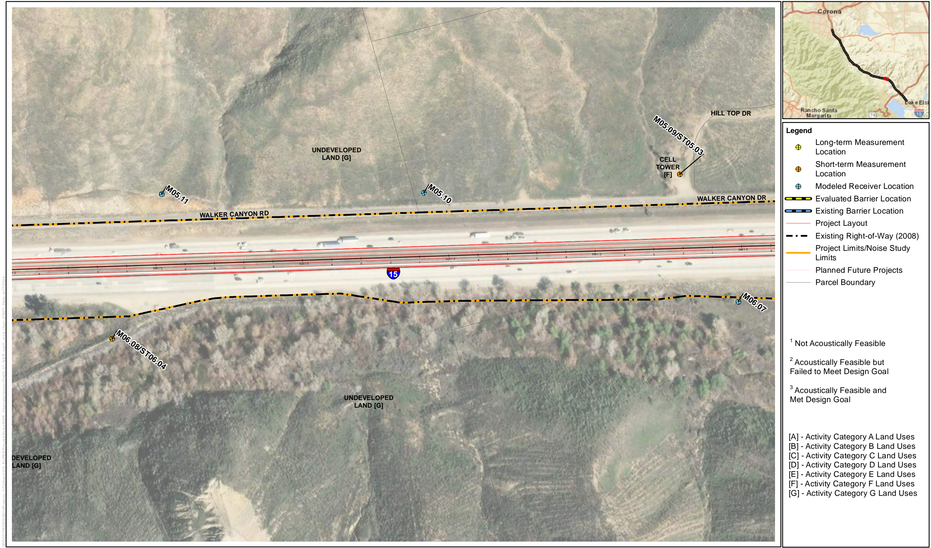
Figure 5-1, Sheet 12 of 40 Noise Measurement and Modeling Locations, and Evaluated Noise Barriers Interstate 15 Express Lanes Project Southern Extension
