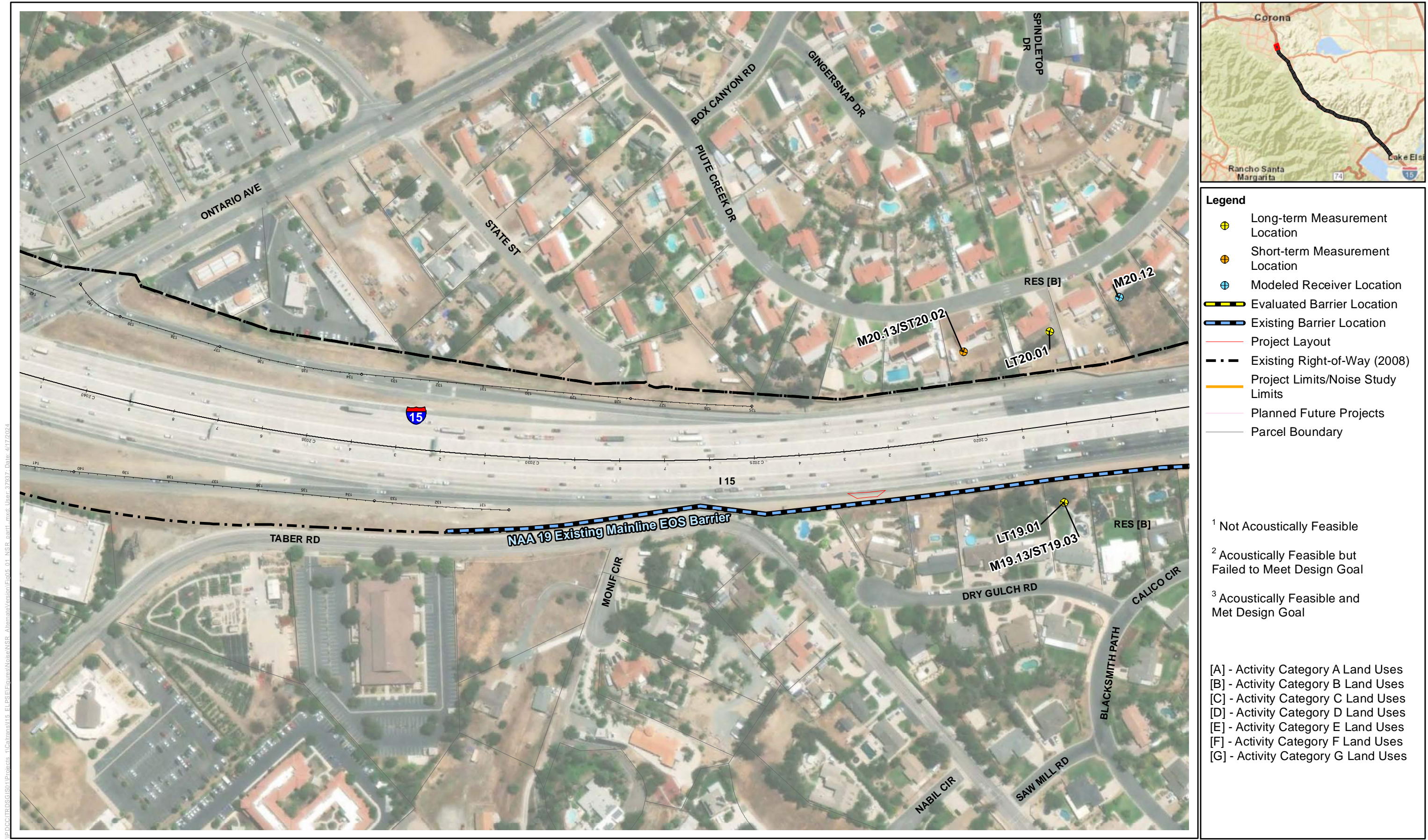
Figure 5-1, Sheet 40 of 40 Noise Measurement and Modeling Locations, and Evaluated Noise Barriers Interstate 15 Express Lanes Project Southern Extension
