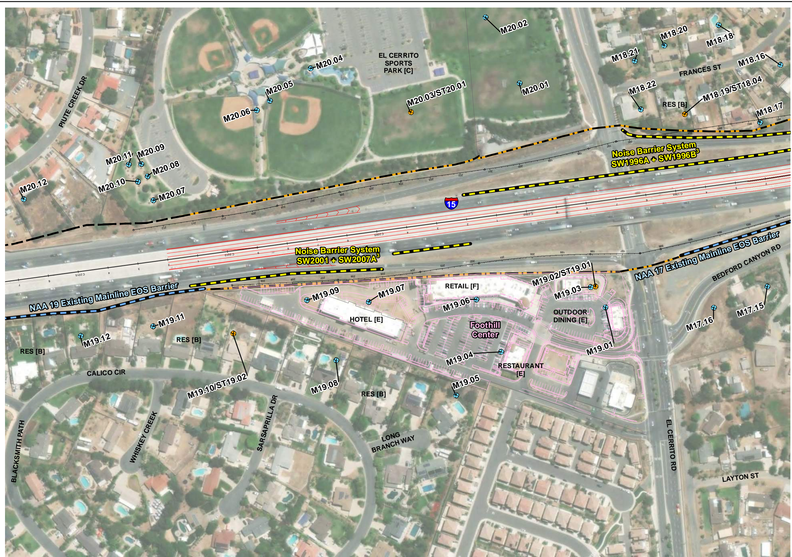
Figure 5-1, Sheet 39c of 40 Noise Measurement and Modeling Locations, and Evaluated Noise Barriers Interstate 15 Express Lanes Project Southern Extension
