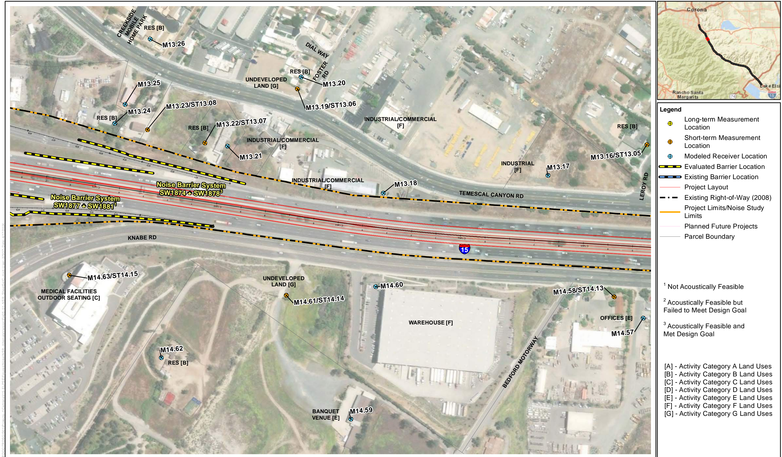
Figure 5-1, Sheet 33c of 40 Noise Measurement and Modeling Locations, and Evaluated Noise Barriers Interstate 15 Express Lanes Project Southern Extension
