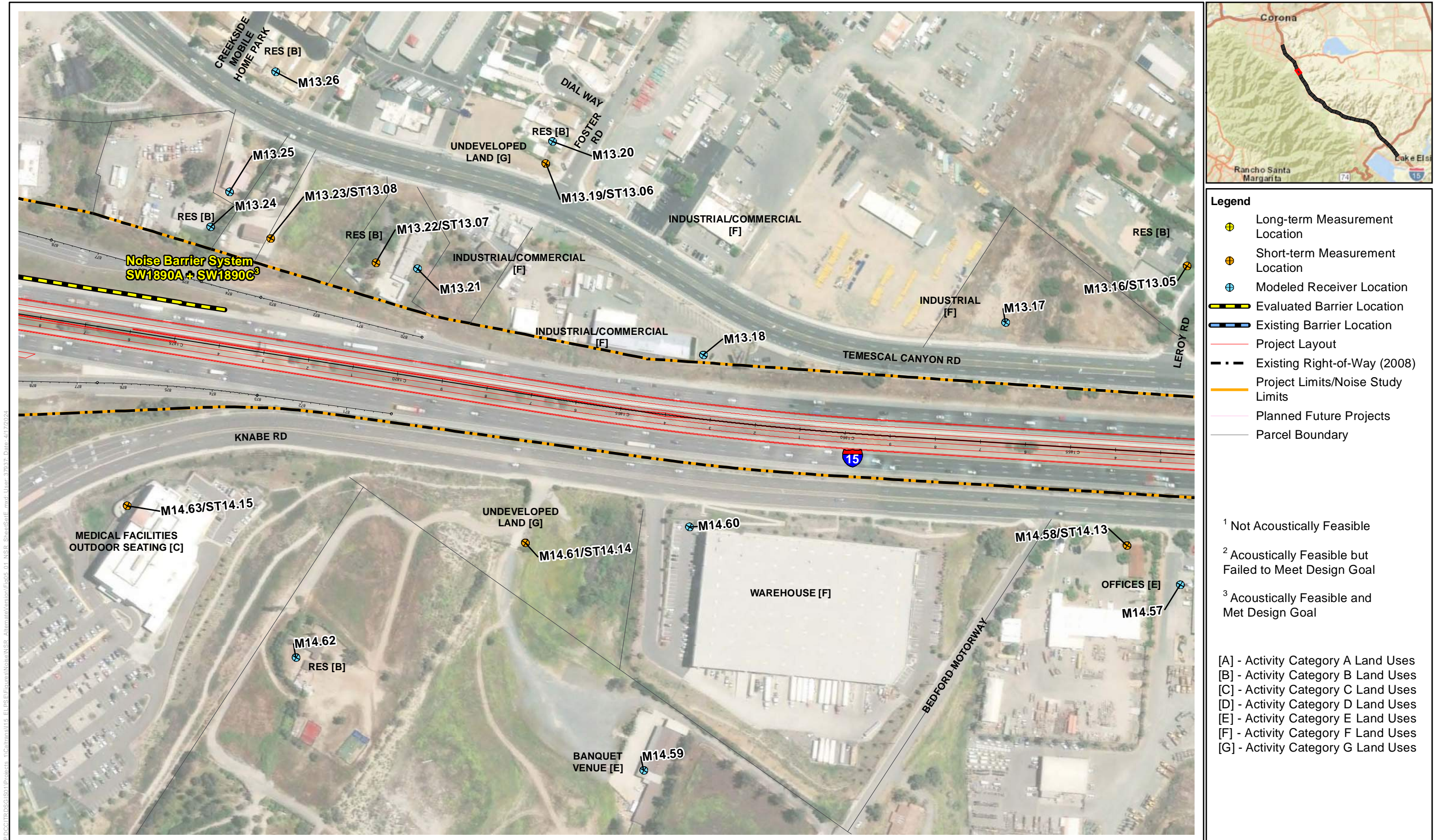
Figure 5-1, Sheet 33e of 40 Noise Measurement and Modeling Locations, and Evaluated Noise Barriers Interstate 15 Express Lanes Project Southern Extension
