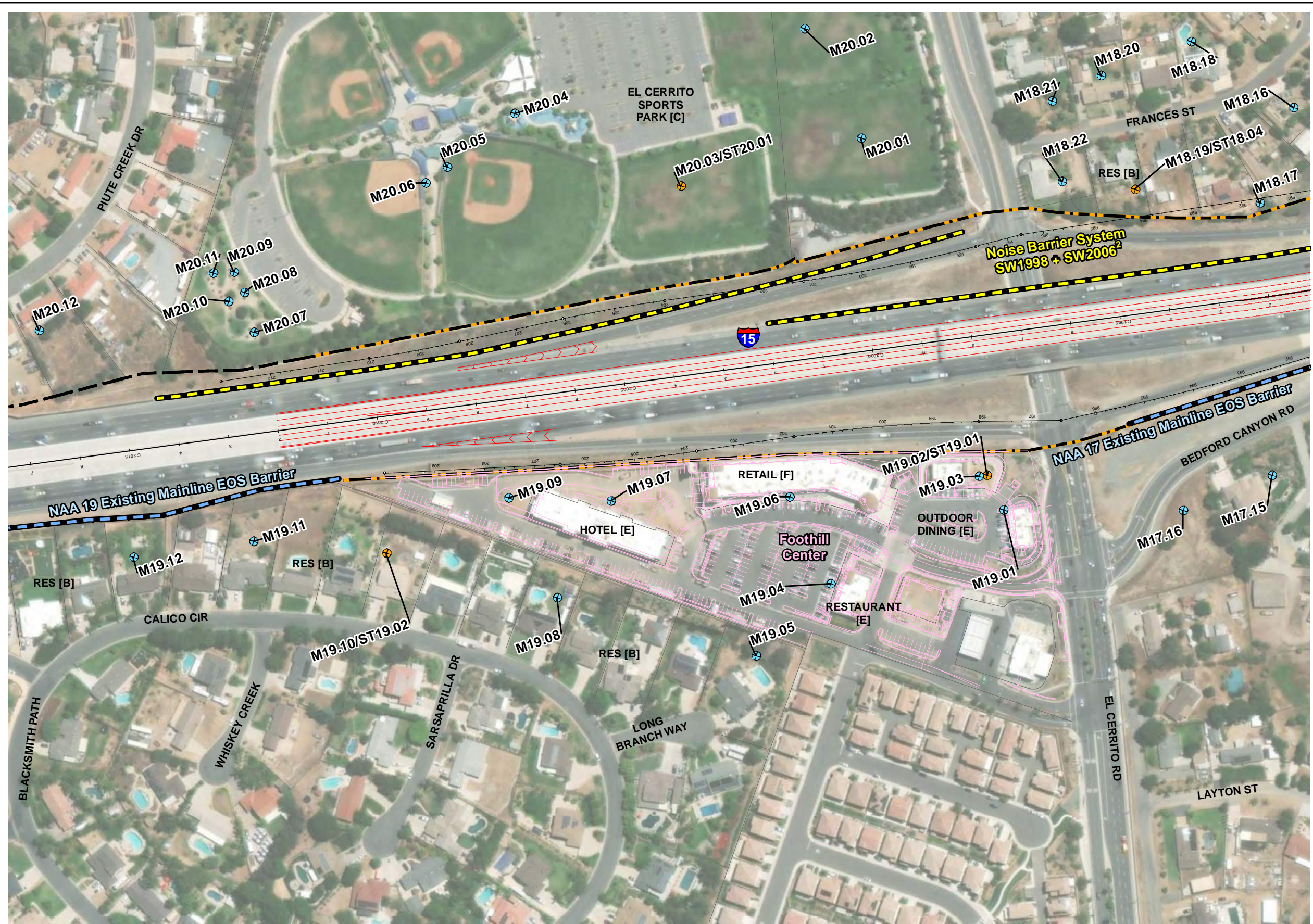
Figure 5-1, Sheet 39d of 40 Noise Measurement and Modeling Locations, and Evaluated Noise Barriers Interstate 15 Express Lanes Project Southern Extension
