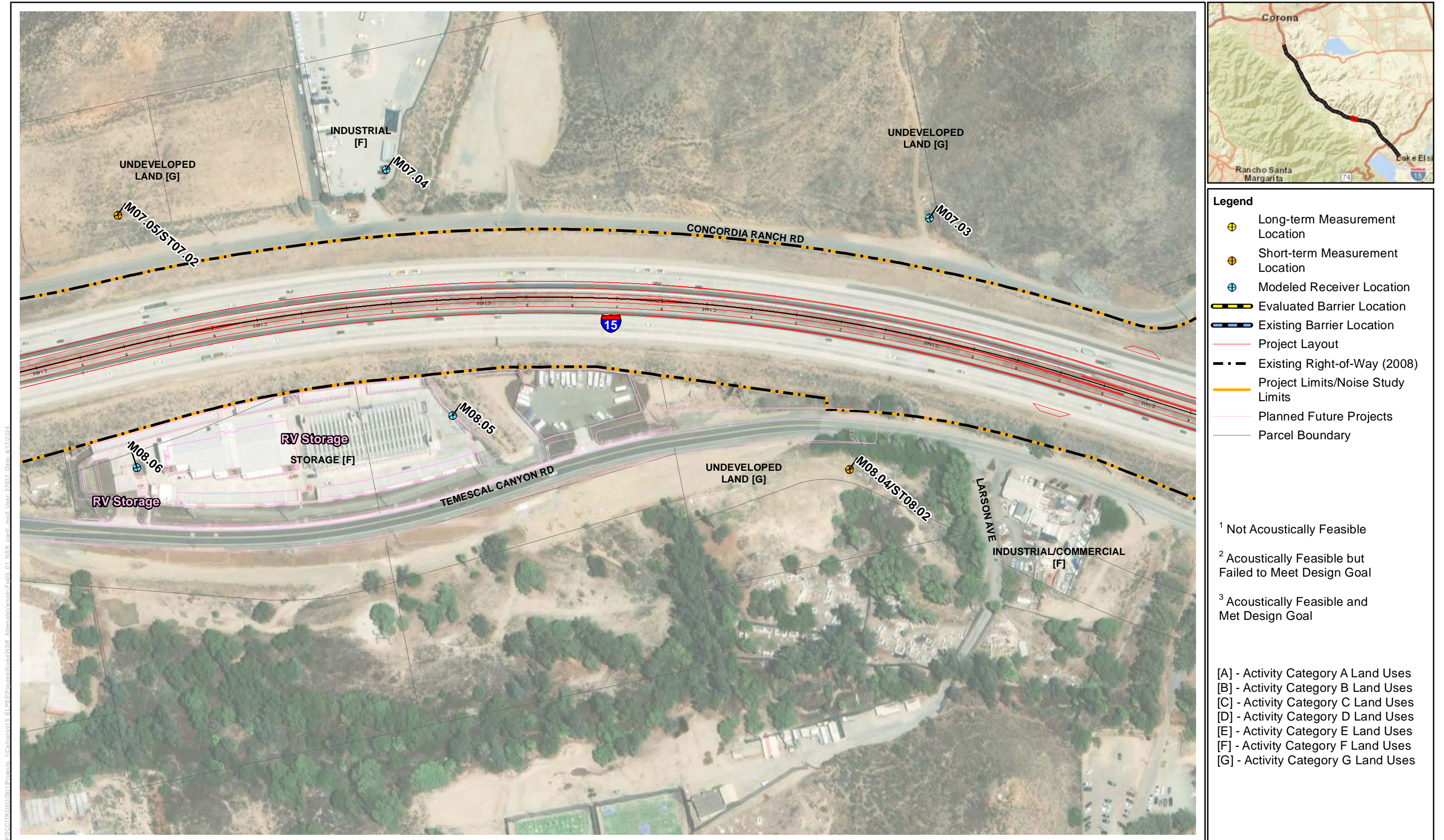
Figure 5-1, Sheet 15 of 40 Noise Measurement and Modeling Locations, and Evaluated Noise Barriers Interstate 15 Express Lanes Project Southern Extension
