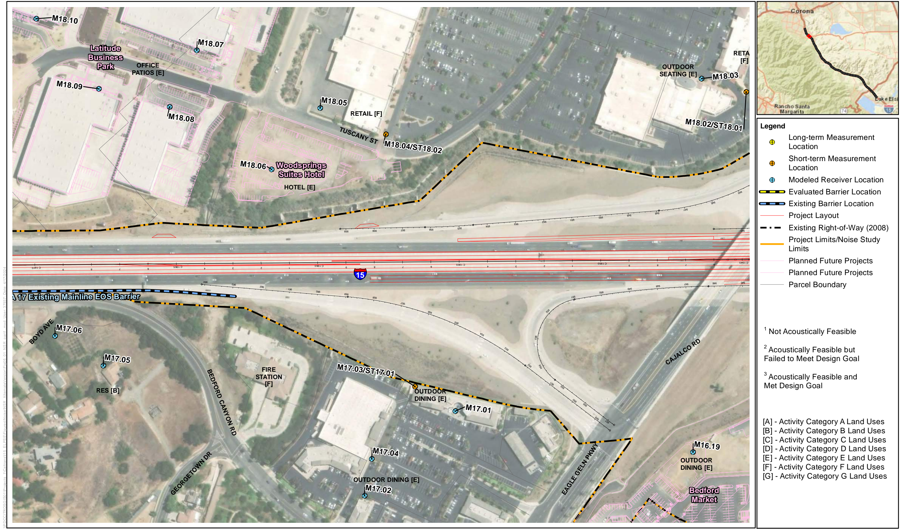
Figure 5-1, Sheet 37 of 40 Noise Measurement and Modeling Locations, and Evaluated Noise Barriers Interstate 15 Express Lanes Project Southern Extension
