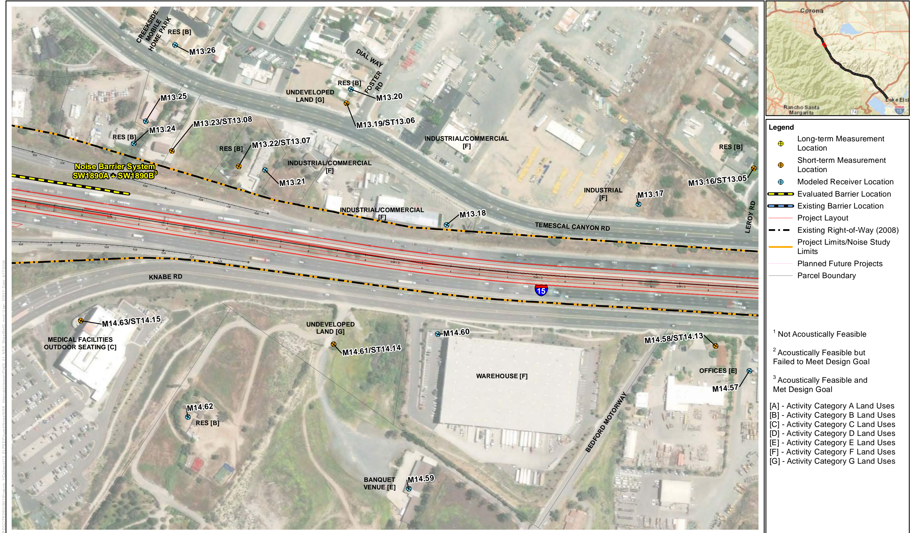
Figure 5-1, Sheet 33d of 40 Noise Measurement and Modeling Locations, and Evaluated Noise Barriers Interstate 15 Express Lanes Project Southern Extension
