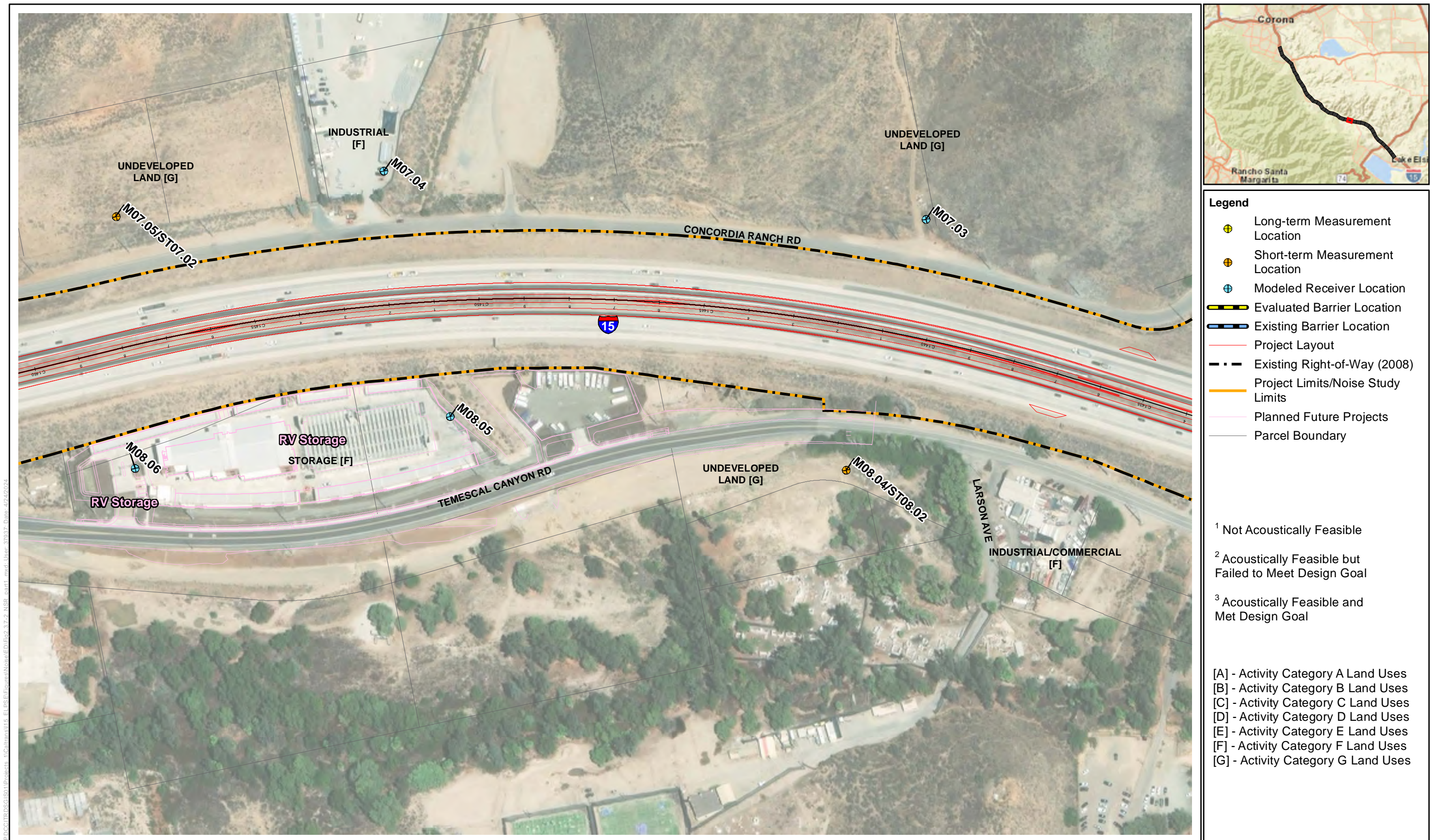
Figure 2.3.7-2, Sheet 15 of 40 Noise Measurement and Modeling Locations, and Evaluated Noise Barriers Interstate 15 Express Lanes Project Southern Extension
