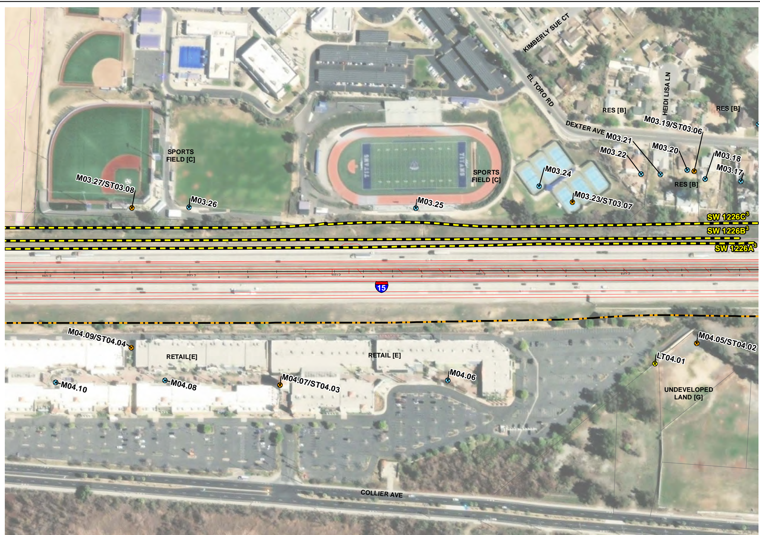
Figure 2.3.7-2, Sheet 6b of 40 Noise Measurement and Modeling Locations, and Evaluated Noise Barriers Interstate 15 Express Lanes Project Southern Extension
