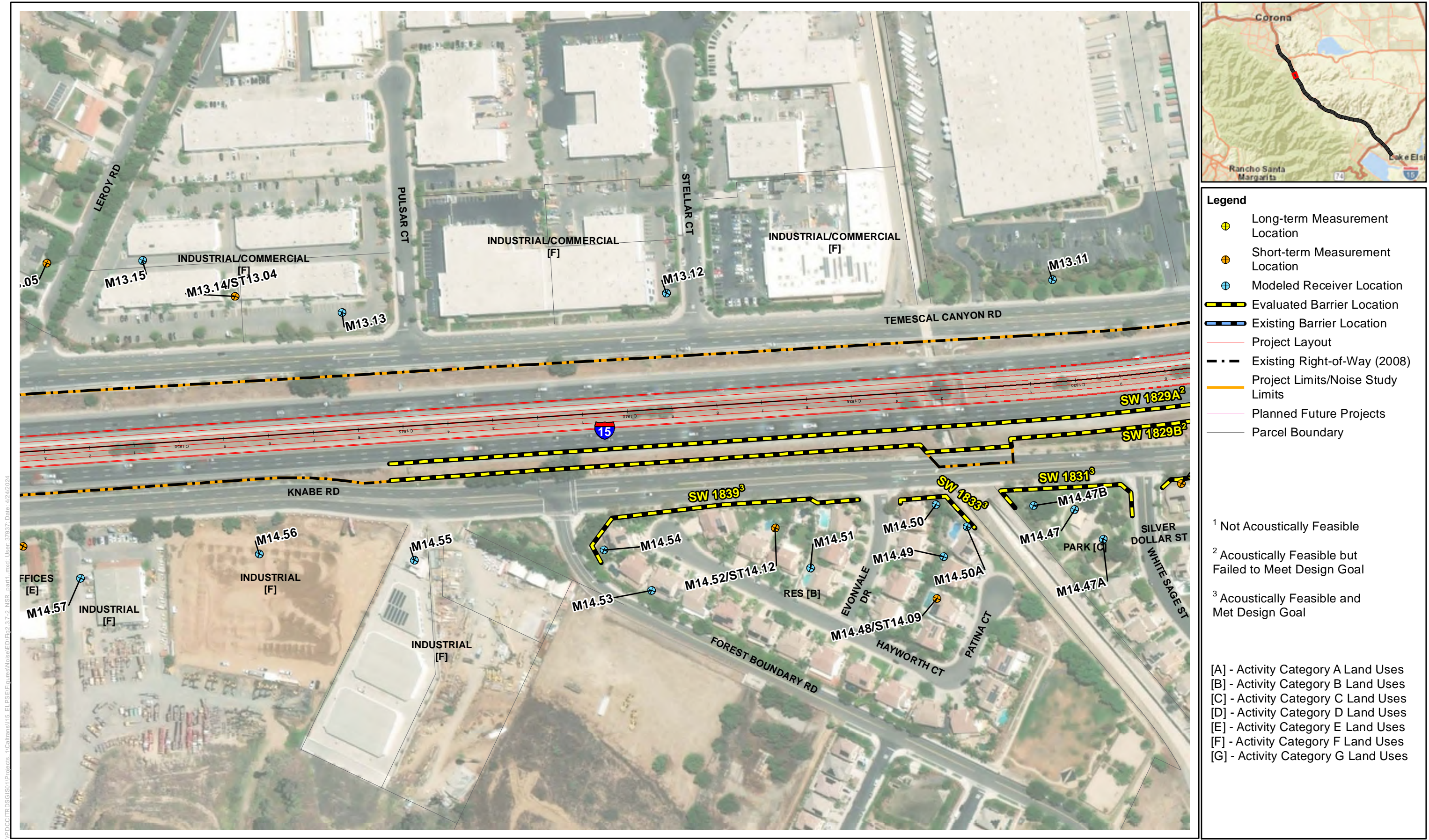
Figure 2.3.7-2, Sheet 32 of 40 Noise Measurement and Modeling Locations, and Evaluated Noise Barriers Interstate 15 Express Lanes Project Southern Extension
