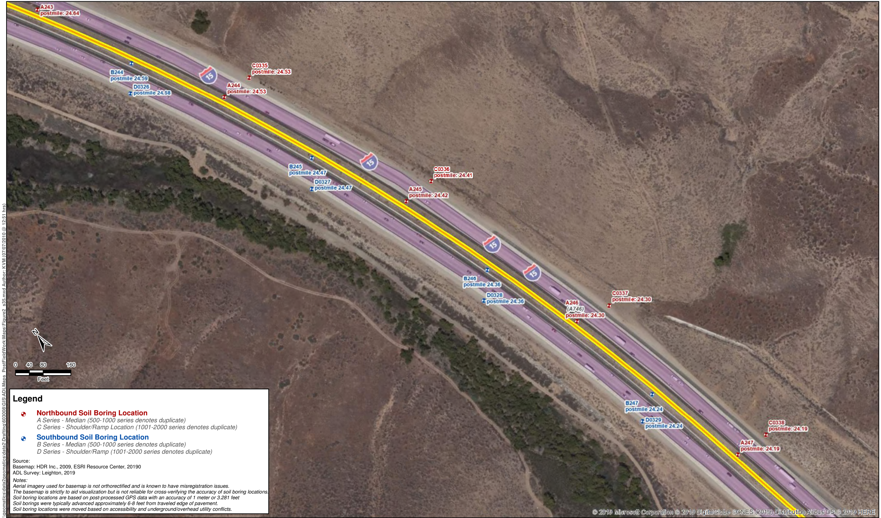
Figure 2 (s10) Boring Location Map, Aerially Deposited Lead Survey I-15 Corridor Improvement Project, Riverside County, California
