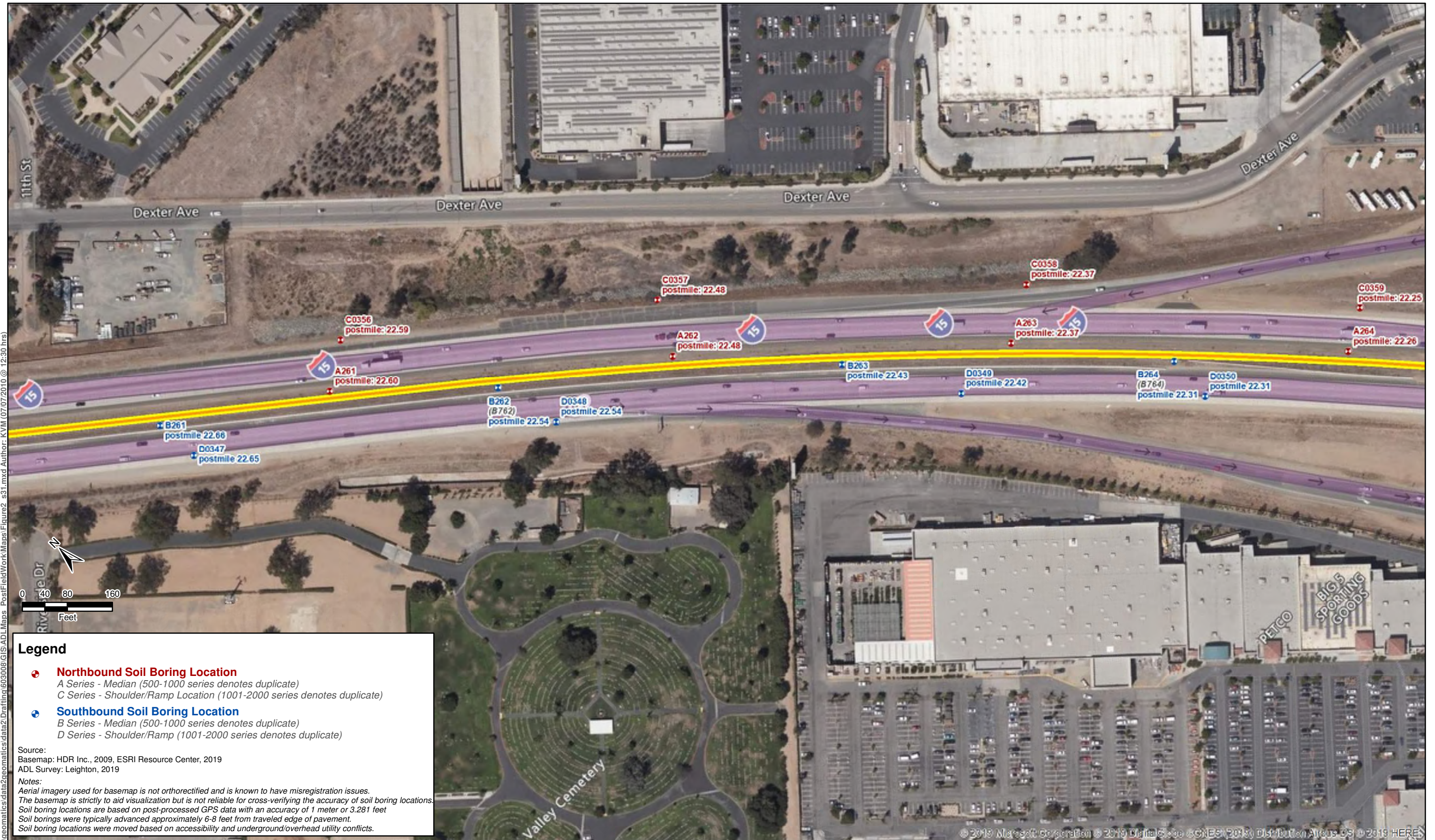
Figure 2 (s6) Boring Location Map, Aerially Deposited Lead Survey I-15 Corridor Improvement Project, Riverside County, California
